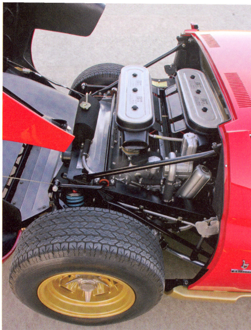
This iteration of the 4.0L Lamborghini V-12 was rated at 385 horsepower, thanks to revised cam profiles. Rear Pirellis made of unobtainium.
