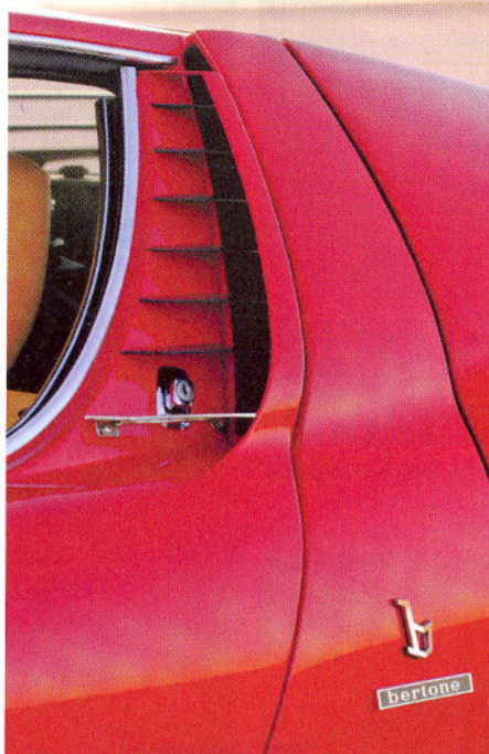
Miura's combination door latch/vent decoration is a clever and subtle styling solution.
